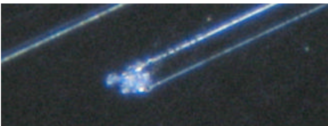
These scratches originated where a moving scraper encountered a fabricating debris defect. Scrapers do not scratch glass.
